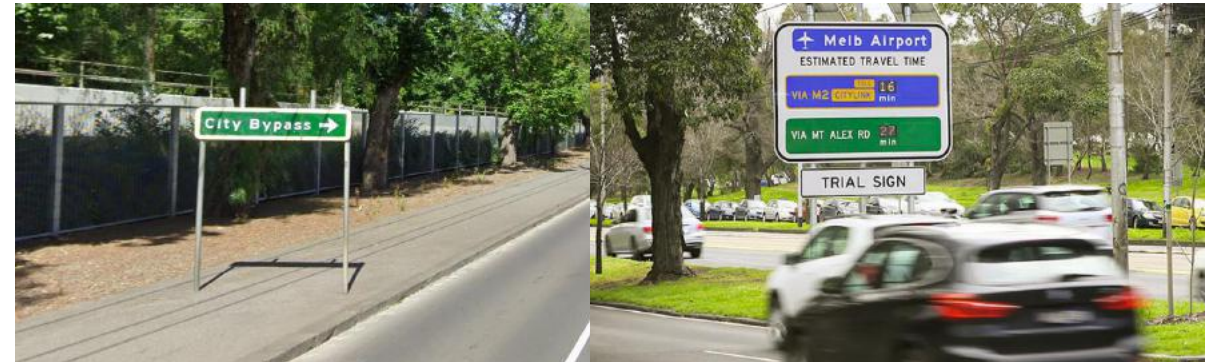
Figure 22: Static and dynamic signage to direct vehicle flows onto preferred and more efficient routes
