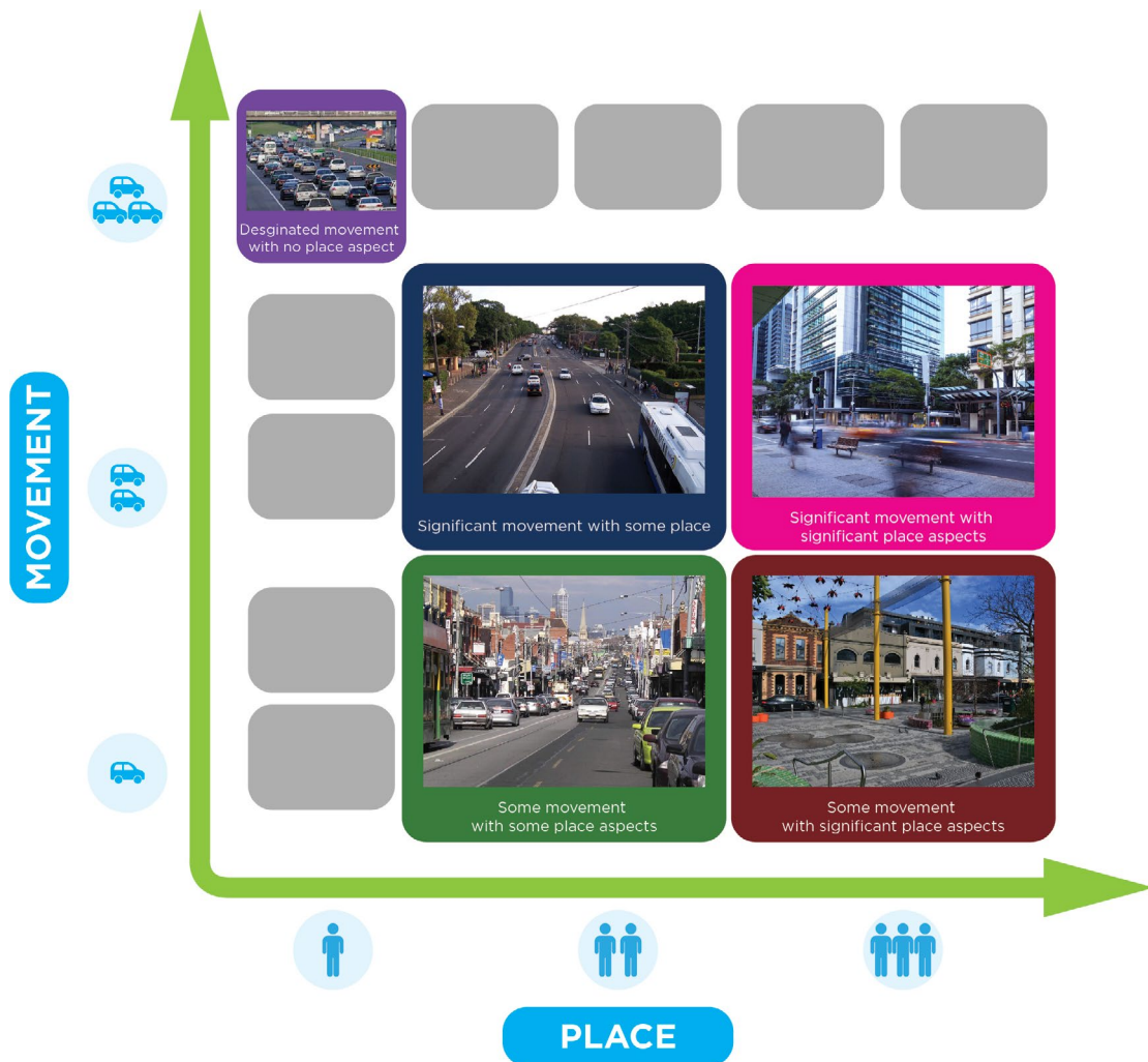
Figure 2 - Example of the Movement and Place matrix. Modified from the Government of South Australia’s ‘Streets for people’ report, as documented in Wooley et al 8 .
