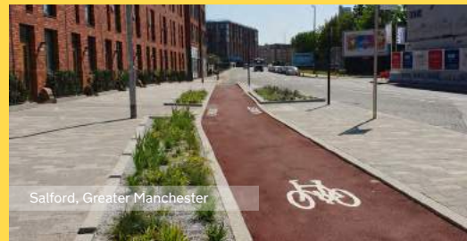
Figure 21. Example of a SUDS segregated cycle track
